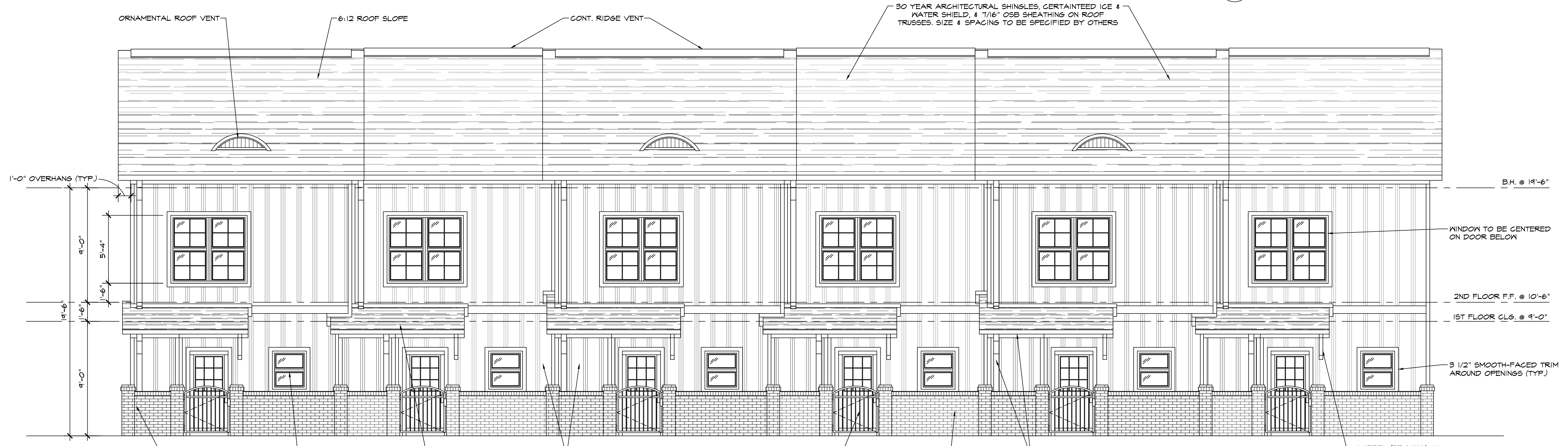
1 FRONT ELEVATION SCALE 1/4"=1'-0"
